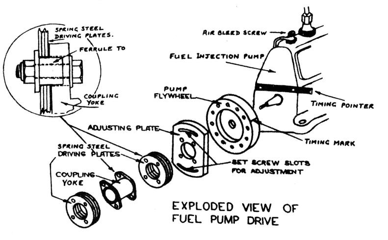
Examine the timing mark pointer on the engine and if bent or damaged repair or straighten as necessary. If the pointer is missing or irreparable the pump will have to be spill timed. Only rarely should spill timing be necessary so details will not be included here but should details be required instructions can be found in diesel engine manuals or alternatively advice can be sought from the technical team on 00-31261.
