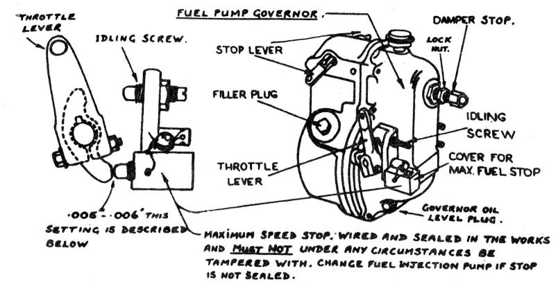
4. Ensure air system is charged. Remove throttle motor cover. Select first throttle speed and check that the engine speed is within the range 550-560 r.p.m. without a tendency to run away.
