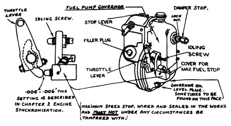
The next job is the governor damper. Remember, this is NOT the means of adjusting engine idling speed and must not be used as such. On the end of the damper screw is a spring loaded plunger which bears on the end of the injection pump rack to stabilise it as idling speed and stop the engine hunting.
